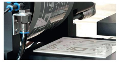
Photo: A newly printed substrate using gravure
